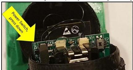
3. Carefully, tuck the solar power wires back in the lid and close the Spike.
